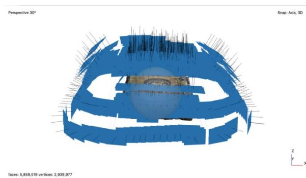
Figure 2. Camera positions and frames on the front and the sides of the icon (processed in Agisoft Metashape Pro)
