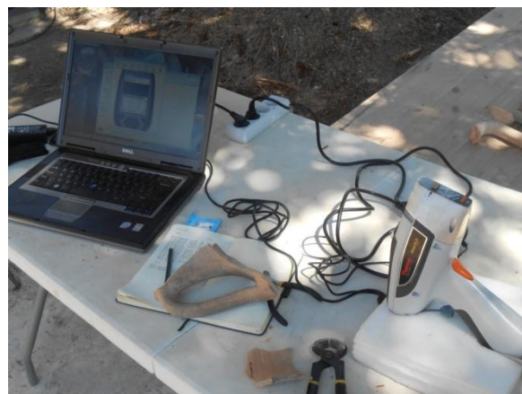
Figure 1 – On-site pXRF measurement of amphora fragments.
