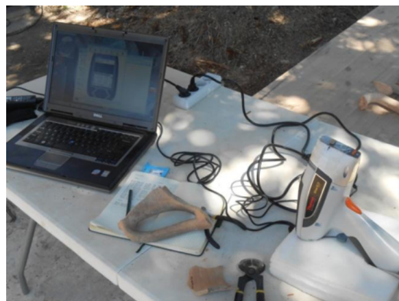
Figure 1 – On-site pXRF measurement of amphora fragments.
